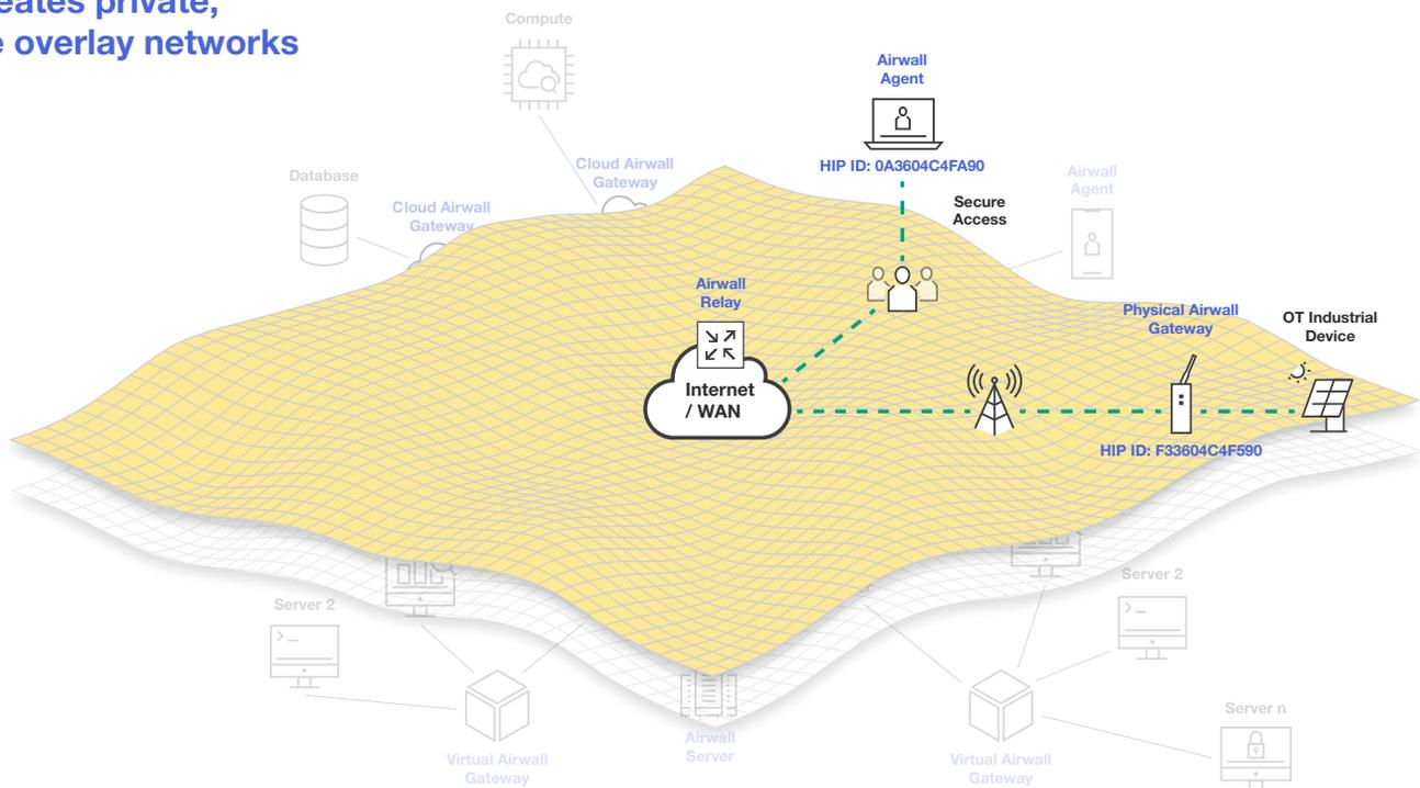
HIP also introduces a new cryptographic host identifier separate from the usual IP address. The fact that IP addresses include both routing/location information and host IDs has complicated security policy management for decades. This new HIP ID allows for simplified, centralized management of end-point access control policies – without the need to change all the access control lists each time a device moves from one location to another.
